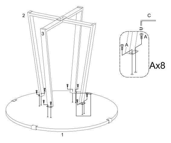
Attach part(2,3) to part (1) using bolt (A) with hex key(C)
