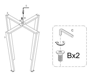
Attach part(3) to part (2) using bolt (B) with hex key(C)
