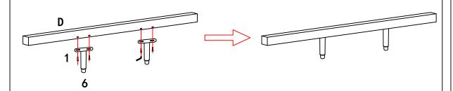
a:Use the Big Screw①to secure the Adjustable support feet 6to the Middle Slat\[D]
