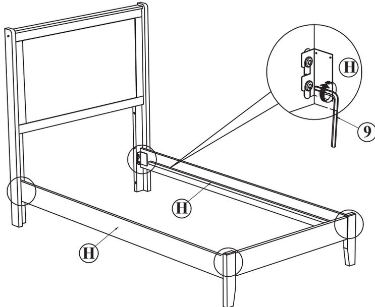
**STEP 6 :** Tighten the 4 Corner with Allen Key (9). Install the bed slat ( G ) to side rail ( H ) and tighten with Csk Screw ( 1 ) as per diagram shown. (NOTE: THE SETUP MUST DONE AT THE DECIDED LOCATION FOR THE BED TO OBTAIN PERFECT STABILITY)
