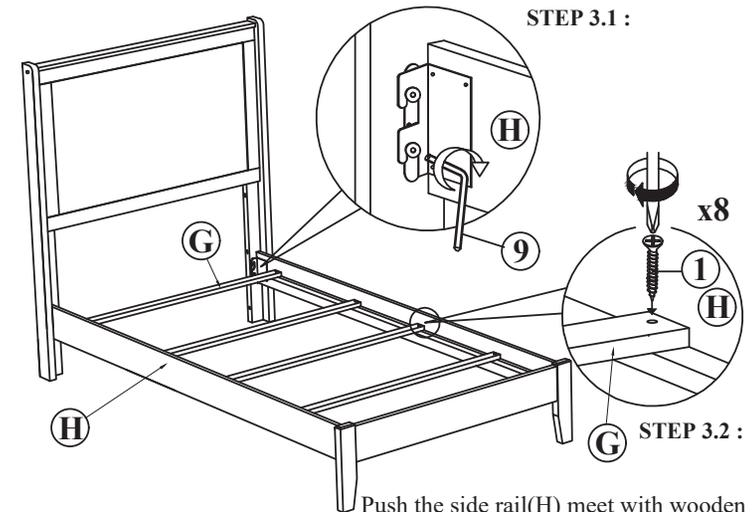
Push the side rail(H) meet with wooden slat(G) and fix the CSK screw (1) by using the Screw Driver.
