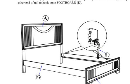
STEP 3: Tighten the 4 Corner with Allen Key (6). Fix the Bed Slat Support Leg (F), to Bed Slat (E) as shown. Install the bed slat (E) to side rail (G) and tighten with Csk Screw (5) as per diagram shown. (NOTE: THE SETUP MUST DONE AT THE DECIDED LOCATION FOR THE BED TO OBTAIN PERFECT STABILITY)
