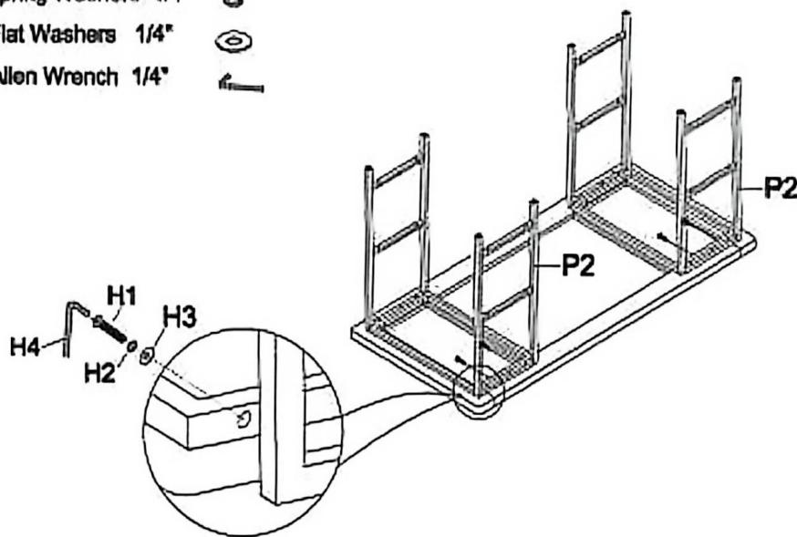
Step 3. Attach bottom shelves (P4) to each leg of side frame (P2), loosely attach all the bolts with Allen wrench (H4) as shown below.
