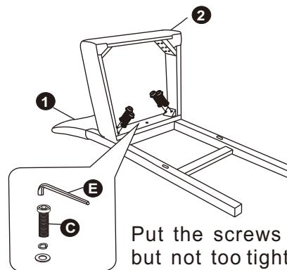
Put the screws in the holes, tight the screws, but not too tight, 90% is ok.
