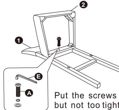
Put the screws in the holes, tight the screws, but not too tight, 90% is ok.
