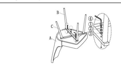
Attach Upper Leg Frame(C) to Lower Leg Frame(B), and Seat(A) using Bolts(1), Spring Washers(2) and Washers(3) with Allen Wrench(4) as shown above. **Tighten the Bolts fully in a sequential manner.**
