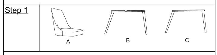
Place the Seat(A), Lower Leg Frame(B), and Upper Leg Frame(C) onto a clean, non-marring surface.
