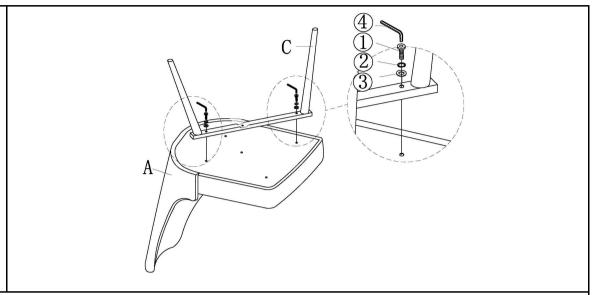
Attach Upper Leg Frame(C) to Seat(A) using Bolts(1), Spring Washers(2) and Washers(3) with Allen Wrench(4) as shown above.
