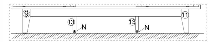
If the TV cabinet is unstable with the ground, please rotate the 13 # adjusting foot pad (N).
