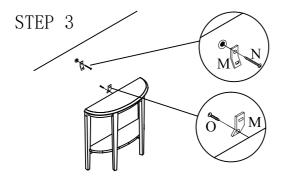
1.Insert drywall screw into metal bracket and into drywall anchor.
