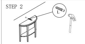
1.Use a light hammer to tap anchor into hole. 2.Anchor should fit snugly.If hole is too small, drill again to increase hole size .Do not force anchor into wall.
