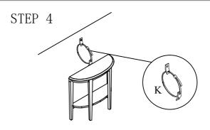
1.Insert strap thru bracket attached to wall. then thru bracket on item, and into head of strap.
